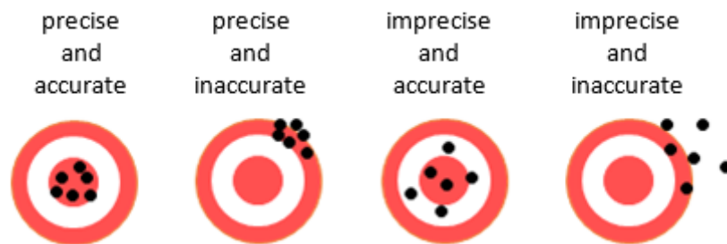
Figure 1-5 Illustration of the difference between accuracy and precision.
