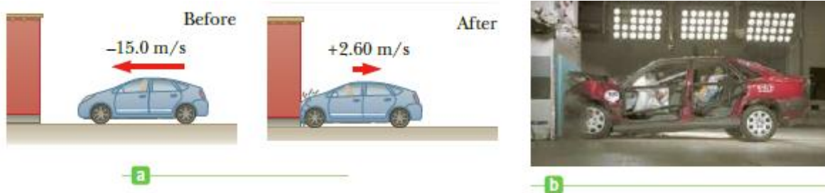
Figure 7-2 Example 7.2) (a) This car's momentum changes as a result of its collision with the wall. (b) In a crash test (an inelastic collision), much of the car's initial kinetic energy is transformed into the energy it took to damage the vehicle
