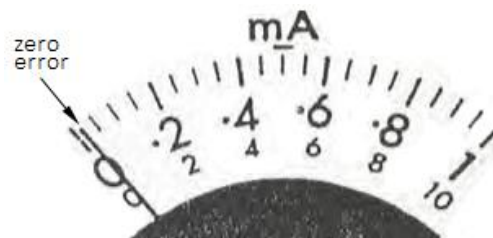
Figure 1-3 The zero error of an ammeter is an example of systematic error
